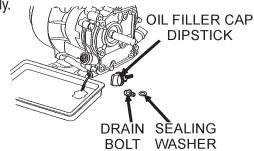
Figure 31. Engine Oil (Draining)
